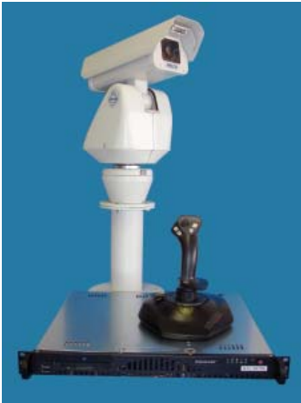
PerceptiVU tracking system with a Logi-Tech Wingman joystick and an optional Pelco Esprit Pan/Tilt unit.
